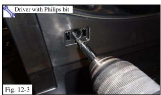
(c) Reinstall the screw at the rear of the cladding (Fig. 12-3).
