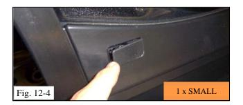
(d) Snap in the small attachment cover at the rear (Fig. 12-4).
